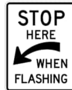
Stop Here When Flashing – for Stop Bars
