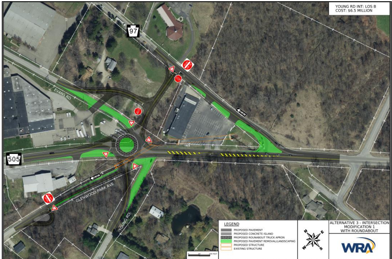
Exhibit ES - 4: Alternative 3 - Intersection Modification 1 with Roundabout
