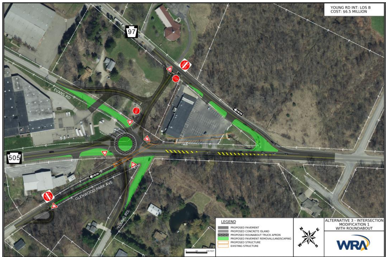
Exhibit 18: Alternative 3 - Intersection Modification 1 with Roundabout
